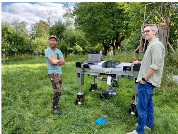
Fence-clearing robot running vegetation-clearing, weed-detection, and bio-mass measurement modules on the same Portainer and AgriGaia backend as the Rumex robots. Images ©Institut für Robotik und Kognitive Systeme, Universität zu Lübeck.
