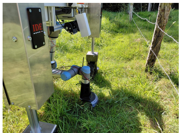
Fence-clearing robot running vegetation-clearing, weed-detection, and bio-mass measurement modules on the same Portainer and AgriGaia backend as the Rumex robots. Images ©Institut für Robotik und Kognitive Systeme, Universität zu Lübeck.
