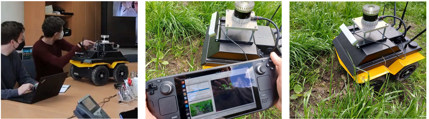
A Clearpath Jackal robot from lab setup to pasture deployment running Rumex weed detection models deployed and kept up to date through Portainer. Images ©Institut für Robotik und Kognitive Systeme, Universität zu Lübeck.
